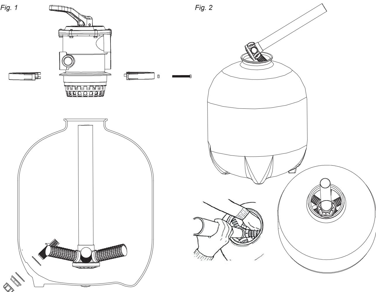
Place the completed manifold on the foundation in the middle of the tank and fill halfway with water to stabilize it. Make sure that the star-shaped gauze is well centralized in the bottom of the filter and that the purge screw is tight.
